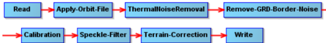
FIGURE 2.3: Standard workflow for processing of Sentinel-1 GRD data.
